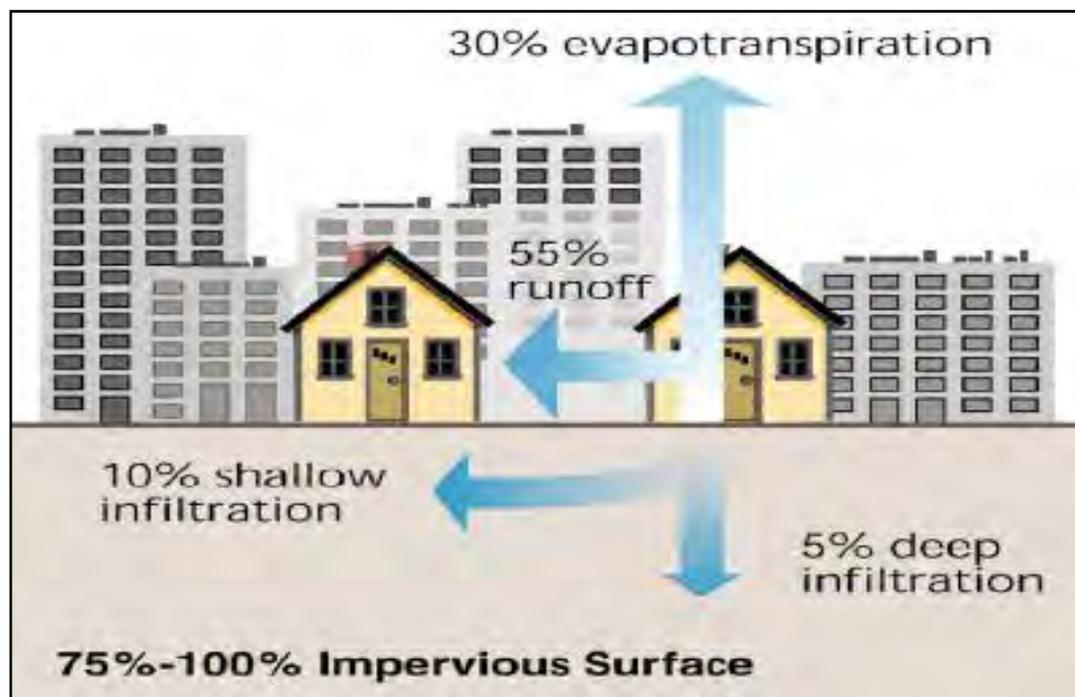
Figure 1. Impervious surfaces in a watershed.
