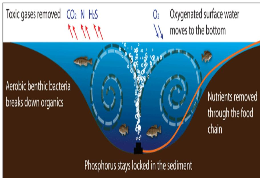
**Figure 37. Diagram of laminar flow aeration. ©RLS**
