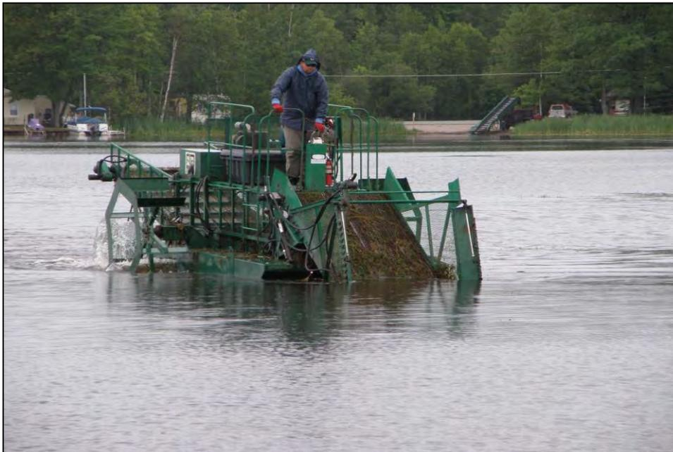
**Figure 33. A mechanical harvester used to remove aquatic plants (RLS, 2018).**
