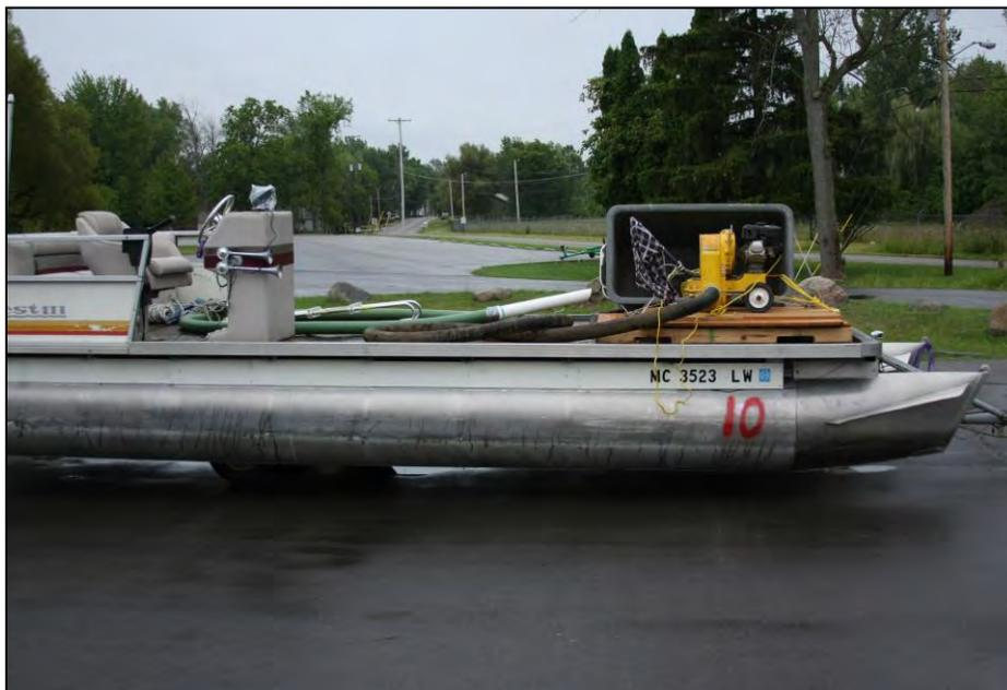
**Figure 36. A DASH boat used for aquatic plant removal (RLS, 2018).**
