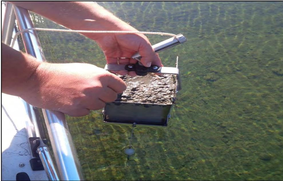
**Figure 24. An Ekman hand dredge for sampling lake sediments (RLS, 2018).**
