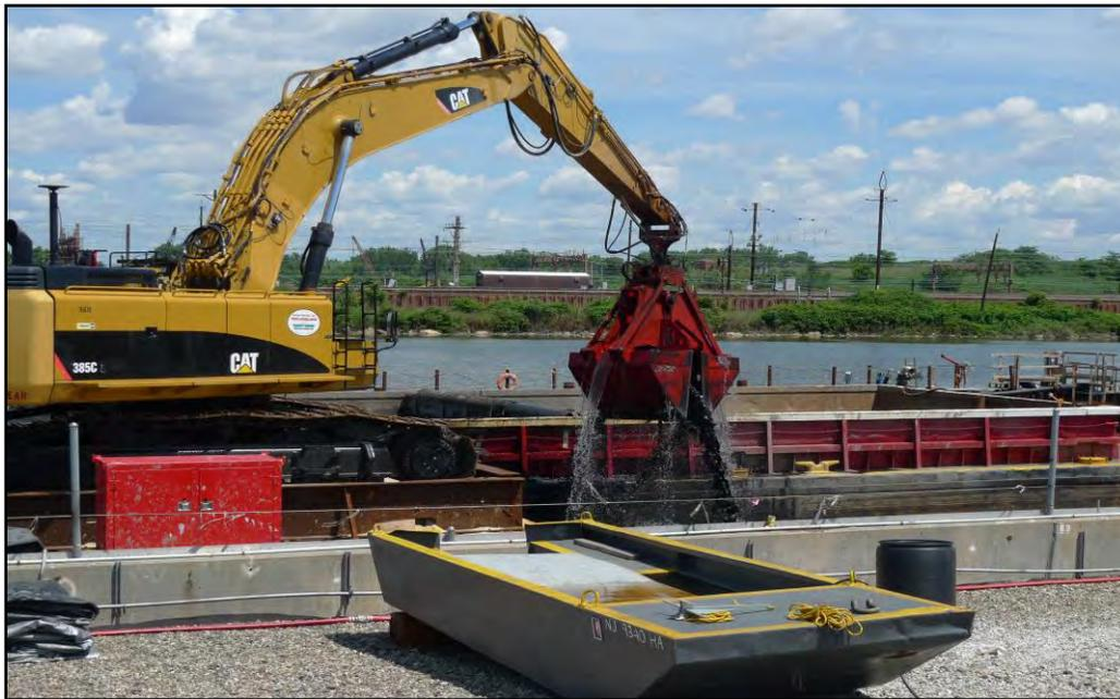
**Figure 38. A mechanical dredge for sediment removal in inland waters.**
