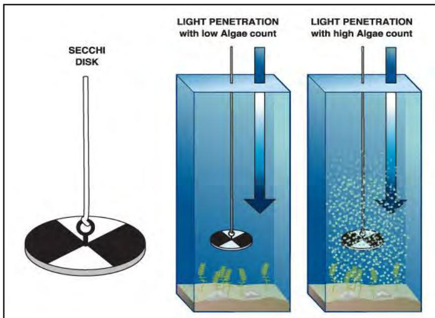
Figure 7. Measurement of water transparency with a Secchi disk.
